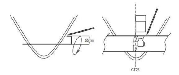
Replace the tunnel. To secure its position apply reinforced fiberglass filler to all areas, both inside and outside, in order to entirely fill the space between the hull and the tunnel. Laminate using a minimum of 8 layers of **ISOPHTALIC RESIN** alternated with mat and roving.
